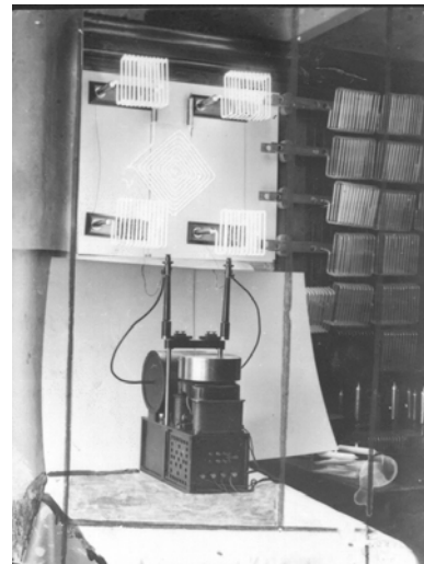
Fig. 5. Tesla's system of glass tubes for low pressure discharge excited by RF source.
